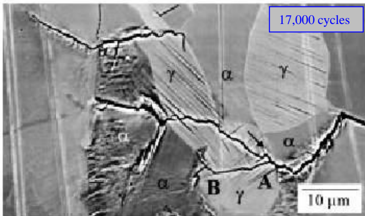
Fig. 6.15 Microcrack propagation in AISI F51 duplex steel during fatigue at \Delta\sigma/2 = 550 MPa (loading axis: \updownarrow ) after (a) 10 500 cycles, (b) 15 000 cycles, (c) 17 000 cycles. (d) Summary of the corresponding crack lengths vs. numbers of cycles data (for details see text).
